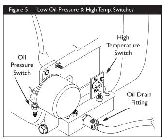
To remedy the low oil pressure condition, fix any obvious oil leak and/or add the recommended oil to the FULL mark on the dipstick. Reset the Fault Detection system as described above.
